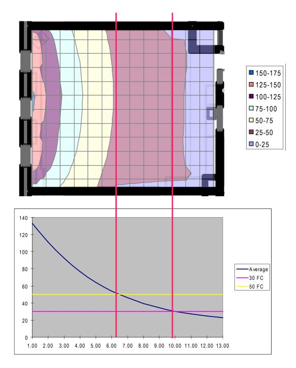
The first floor southeast facing classrooms have a sufficient amount of daylight under clear sky conditions. However the daylighting strategies are for overcast sky conditions. The target luminance of 30-50 fc occurs deep in the space. The graphs above shows glare and contrast in the space.
