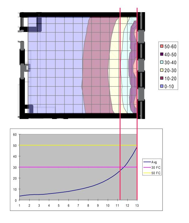
The first floor northwest facing classrooms do not have a sufficient amount of light to effectively daylight the space. The reason being is that there is only a 5% window to floor area ratio. The existing daylight scenario has a lot of glare and contrast. Luminance values drop off steeply at the window wall. The image on the previous page reflects glare and contrast.
