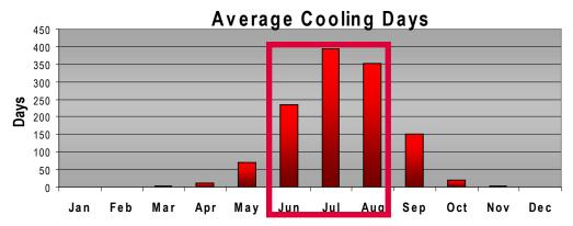
The data shows that there are more heating than cooling days and the cooling days are primarily during the non-occuppied time of the year. Solar heat gain in the winter months is not as much of an issue.
