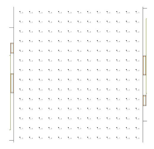
The first floor work areas between the classrooms receive little if any light from the exterior. There is no real feasible way to effectively daylight these spaces. This is due to the distance that these spaces are from the exterior and the amount of glazing on the exterior and interior.
