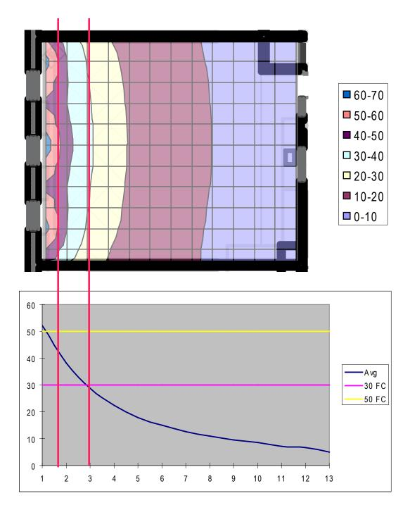
The first floor, southeast facing classrooms do not have a sufficient amount of daylight under overcast sky conditions. The graphs above show that there is a lot of glare. The steeper the curve equals more glare. The image on the previous page shows that there will be large amounts of contrast due to the low window to floor area ratio.
