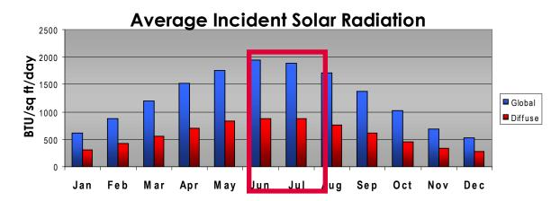
The months with the highest radiation is during the non-occuppied time of the project. However some of the highest radiation is during the heating months of the year. This is a reason for reducing solar heat gain and using low SHGC glazing on overexposed facades.
