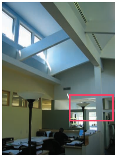
This image shows the location of the IAQ test tube locations and where the dust samples were taken.
