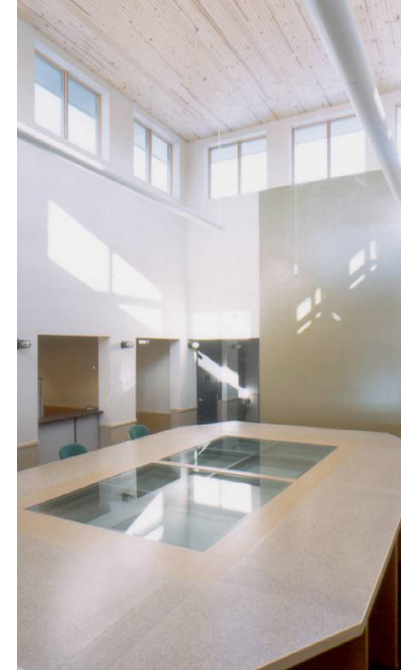
Monitors provide an even distribution of light into the space.
