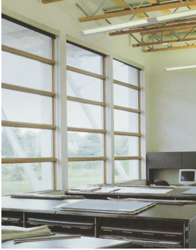
Placement of low-height furniture perpendicular to the window wall allows deeper light penetration into the space.
